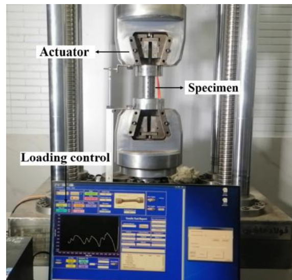
Figure 4: FOLAD MACHINE Hydraulic Testing Machine
